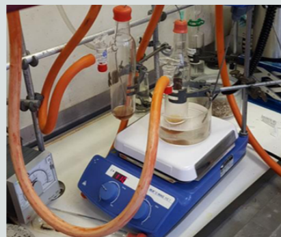
Cannula transfer of air-sensitive materials
